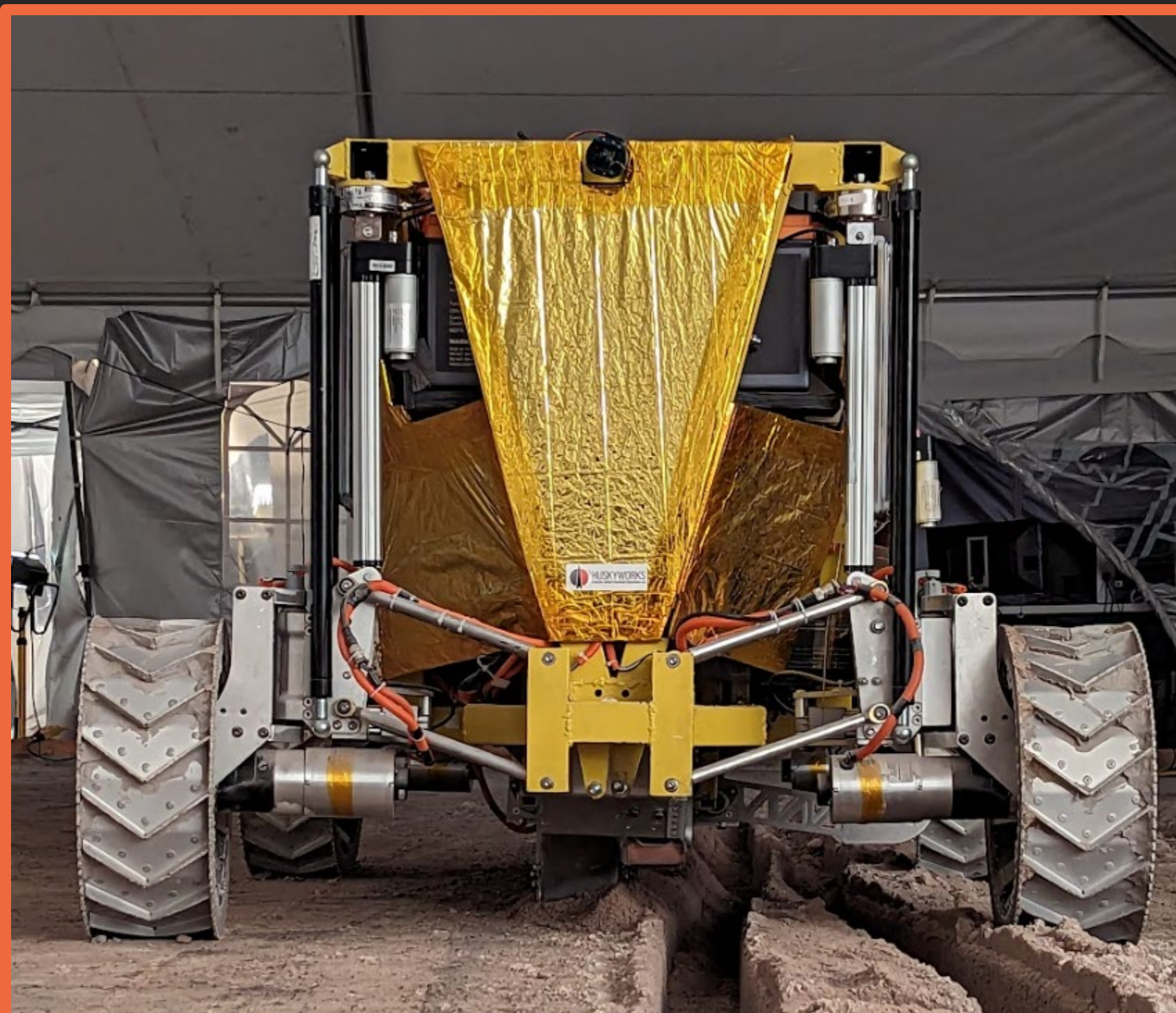
PRIMROSE Excavating Icy Lunar Regolith Simulant
